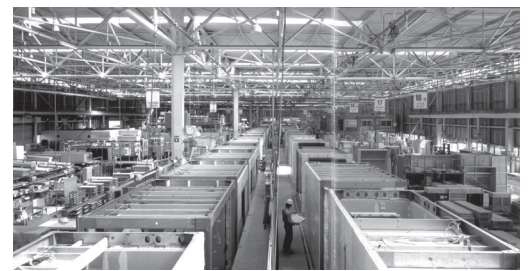
293 Sekisui Heim, housing factory in Japan
